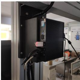
This software is equipped with a special software dongle, the appearance of the dongle is similar to a U disk, should be inserted in the computer USB connection, as shown, the customer should properly save the dongle, if the dongle is artificially damaged or lost, You need to buy a new software dongle.
